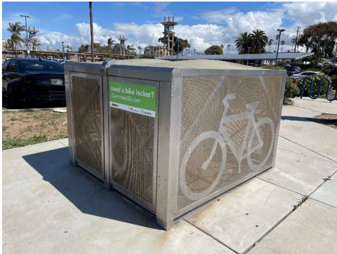
SANDAG Regional Bike Locker Program. This is one Quad Unit (room for 4 bikes total). Bikes access from front and back of unit.
