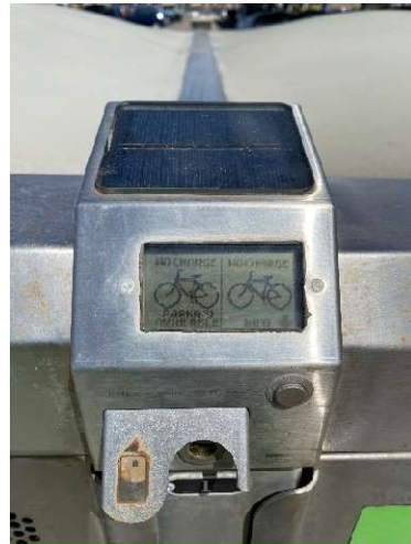
Close-up of solar-powered electronic lock and card reader.
